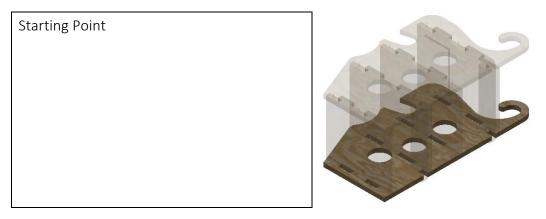
Step 1 Slot Part A in the top slots and Part B in the bottom slots of a Part D Step 2 Slot the Part Cs in the remaining slots of Part D Step 3 Slot the other Part D into the other side of Parts A, B and C Step 4 Slot both of the Part Es into both Part Ds
